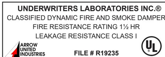
This combination fire/smoke damper meets the construction and performance requirements of:
